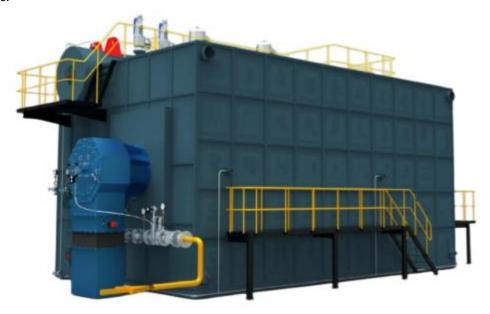
The furnace is surrounded by water-cooled walls. The water-cooled wall usually adopts a membrane wall structure. The membrane-type water-cooled wall on the left side of the furnace completely seals and separates the furnace and the convection tube bundle. The rear part of the convection tube bundle area is a sparse staggered structure (convection tube bundle I zone), and the front part is a sequential structure (convection tube bundle I zone).
