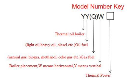
Example:YWQ-1000=YQW series thermal oil boiler,Rated thermal power 1000kw,Fuel gas or oil;Q means gas,Y means oil
