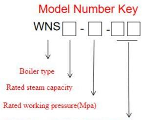
(natural gas, biogas, coke gas, light/heavy oil, methanol, diesel etc.)Fuel
